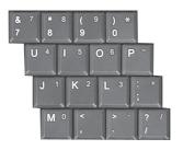
Figure 4: Embedded Numeric Keypad
